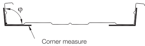
Figure 3.26: Measurement of corner angle flange/web
