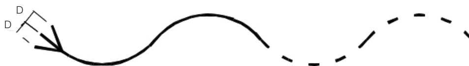
Figure 3.20: Deviation of side lap D
