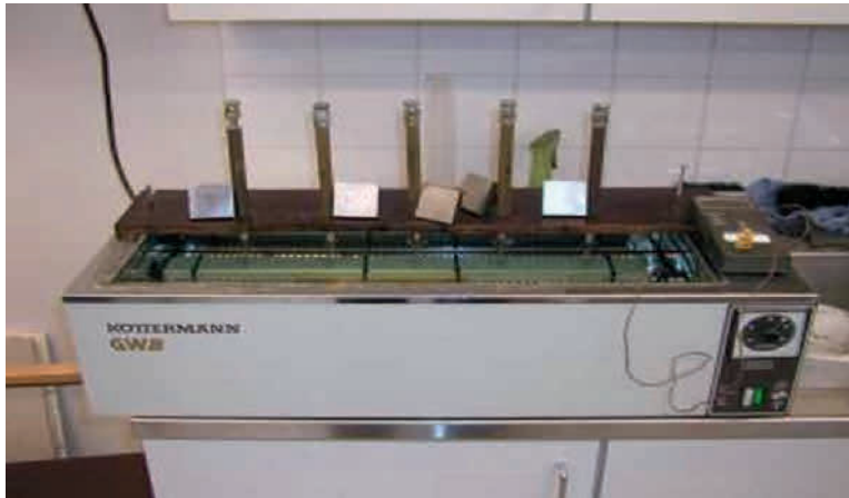
Figure 36: Wedge test arrangement
