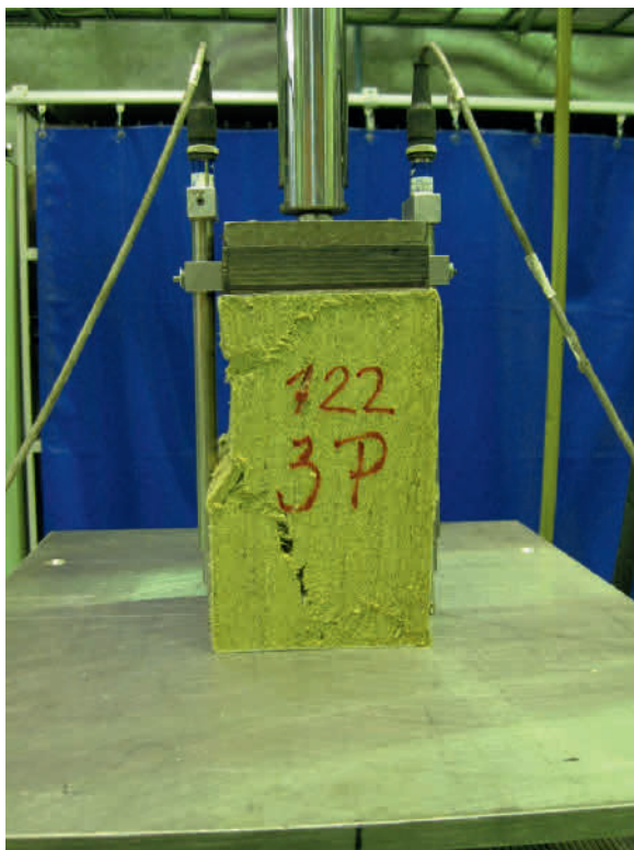
Figure 12: Compression test failed specimen
