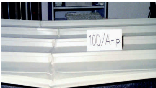
Figure 21: Buckling of the trapezoidal face (positive orientation)
