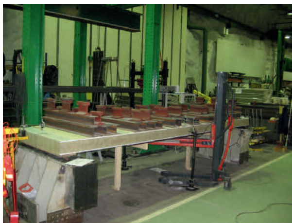
Figure 26: Creep coefficient test set-up
