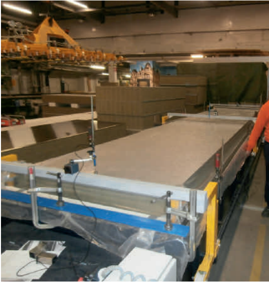
Figure 19: Test set-up in partial vacuum bending test
