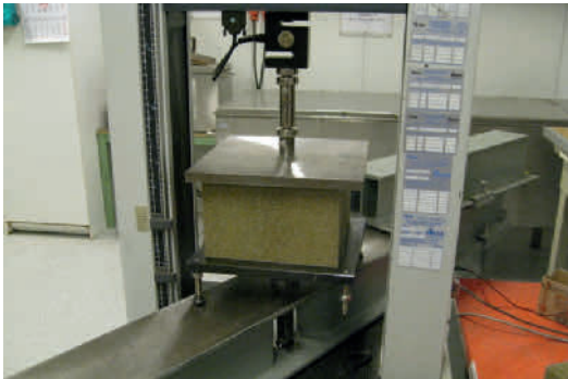
Figure 11: Test of compressive strength and compressive modulus
