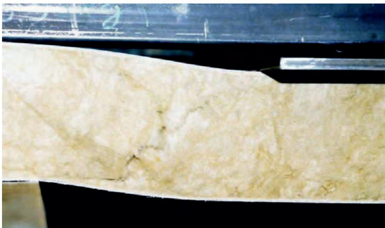
Figure 7: Shear tests on short beams of MW cored panels
