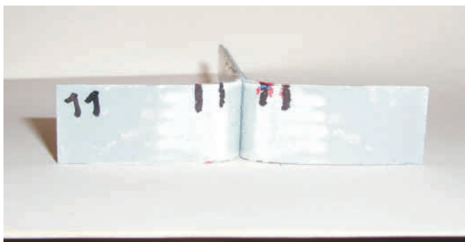
Figure 38: The specimen after exposure (the crack tips are marked on the strips)
