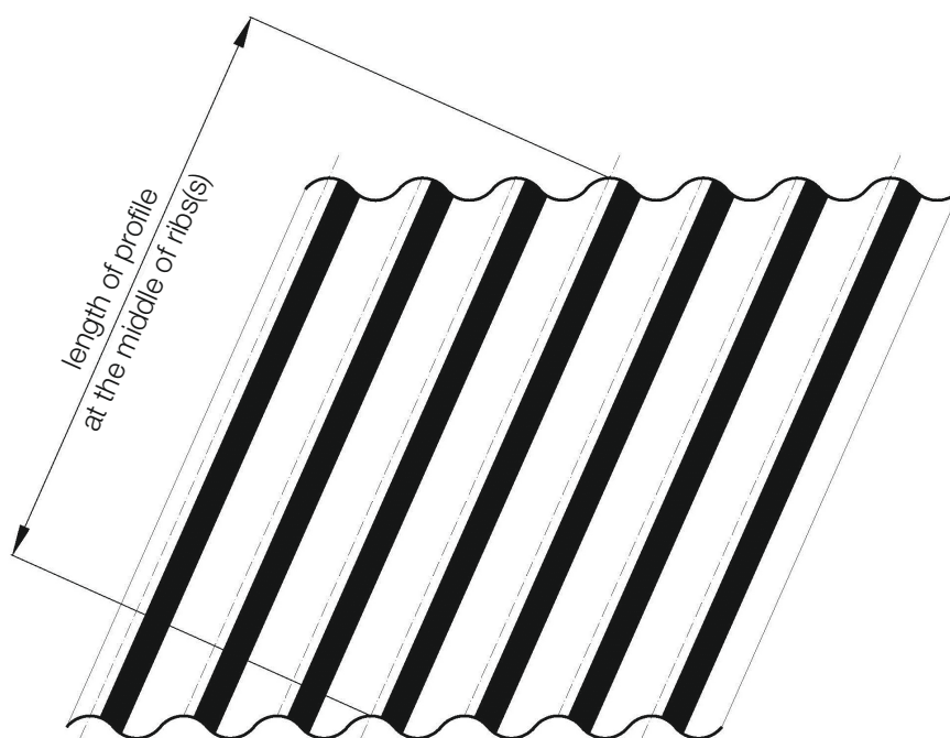
Figure 3.18: Measurement of length of profile at the middle rib(s)
