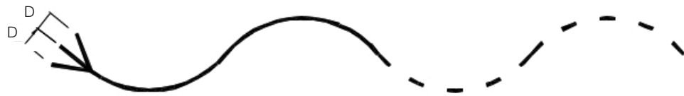
Figure 3.20: Deviation of side lap D
