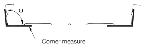
Figure 3.26: Measurement of corner angle flange/web
