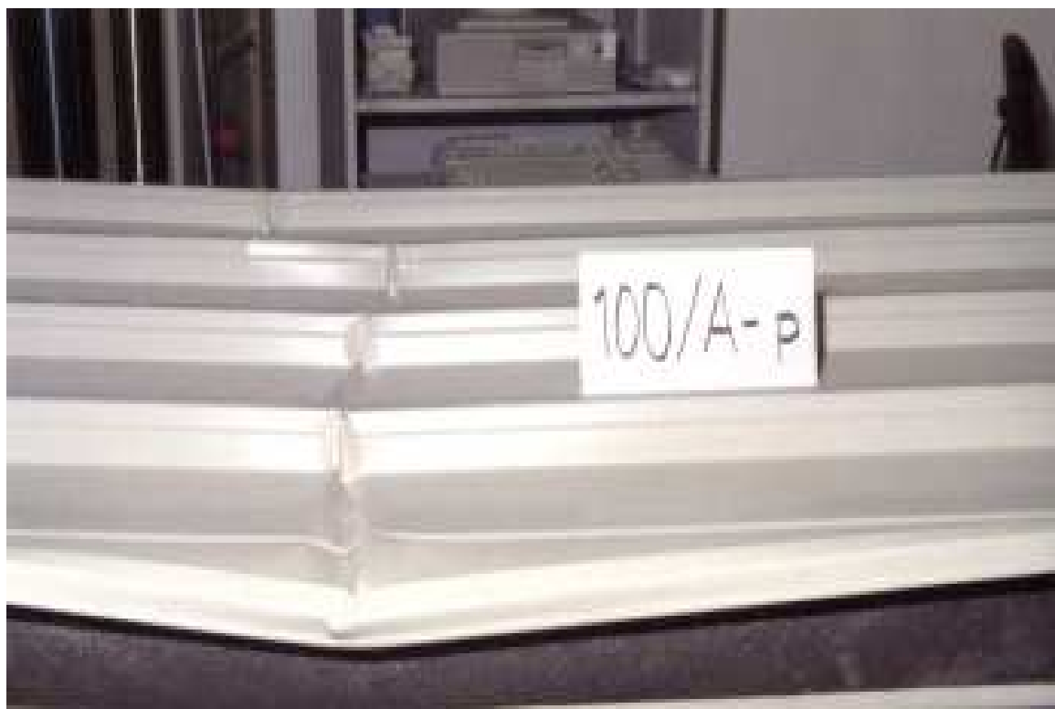
Figure 2.4: buckling of the trapezoidal face (positive orientation)
