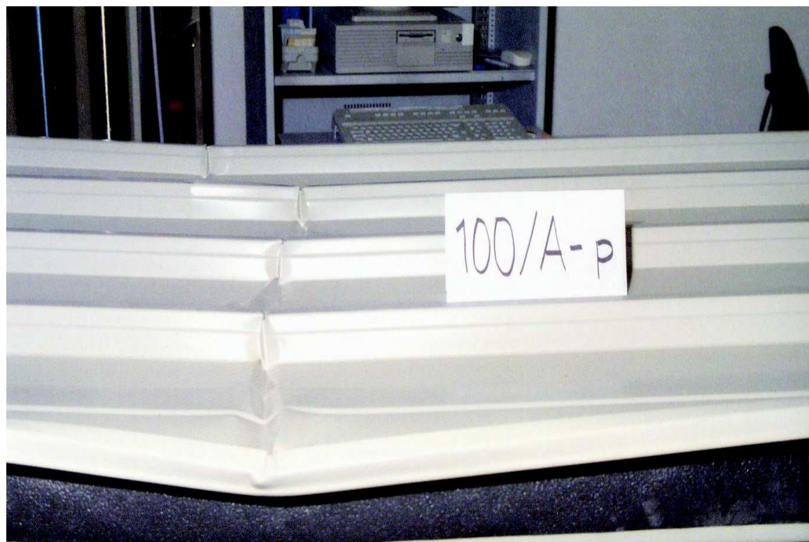
Figure 2.2: buckling of the trapezoidal face (positive orientation)
