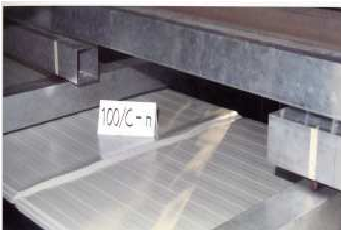
Figure 2.3: wrinkling of a lightly profiled (quasi flat) face (negative orientation)
